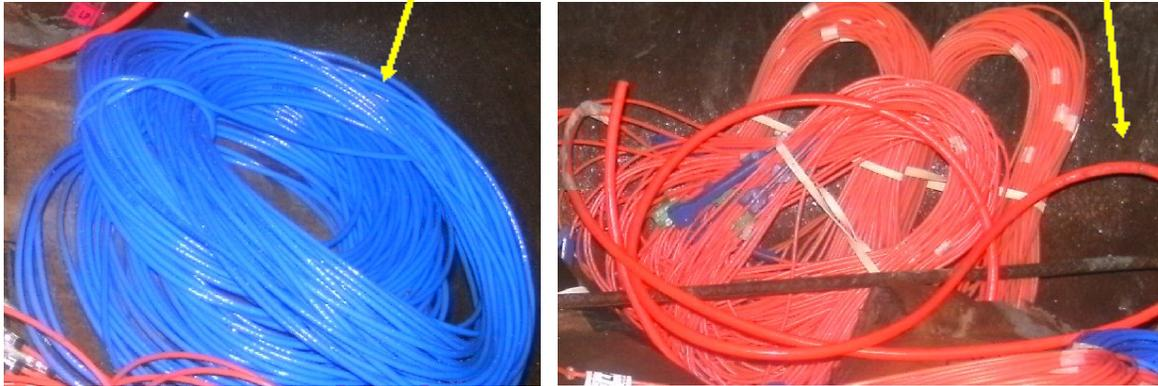
**Figura 16** Detonadores No Eléctricos
